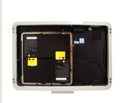
The tablet batteries power both the GETAC tablet as well as the entire Mark IV Tank Floor Scanner. Operators are able to replace one battery at a time with no power interruption to the Mark IV.
